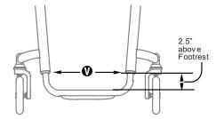
**V-FRONT END v** Measure from <u>inside</u> of front frame tube to <u>inside</u> of opposite front frame tube 2-1/2" above footrest. (Required with Front Seat Taper T. Titanium Footrests have 1" of adjustment up and down. Not available with Ergonomic Seat frames.) ZFE2
